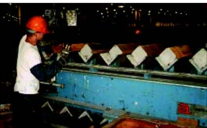
Louisville Forge & Gear Works produces quality precision forgings for high performance use in the automobile, aerospace and farm machinery sectors as well as other markets. Among its better-known products are drive shafts. Part of the process includes setting molds as shown above. Photo provided by Louisville Forge & Gear Works LLC
